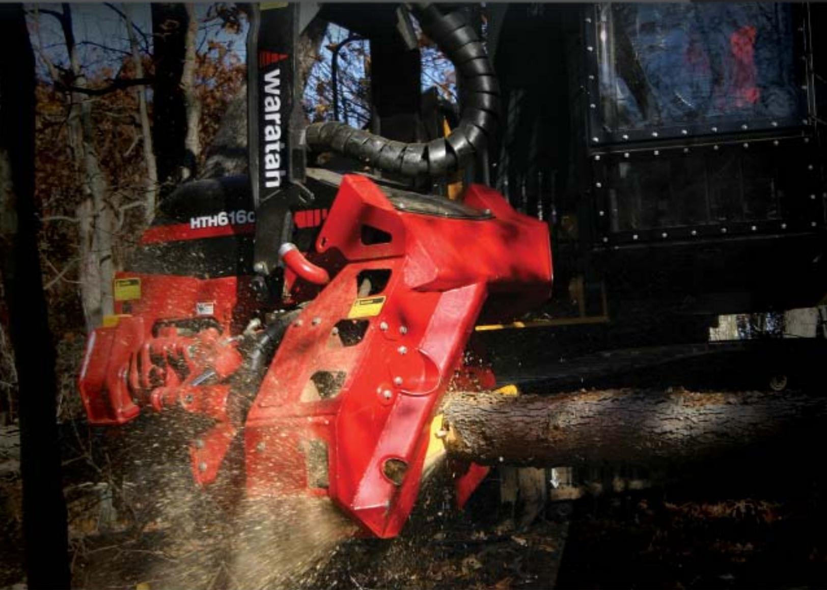
Lightweight and versatile, the HTH616C gives you the same great features you'd expect on larger heads, like a synchronized drive and a topping saw. Use it to process small wood out of a deck, work behind a buncher, or cut and delimb post and rail in a mill yard. It can easily be installed on carriers for thinning and final-felling wood at an optimal 40 centimeters (16 inches) in diameter.
