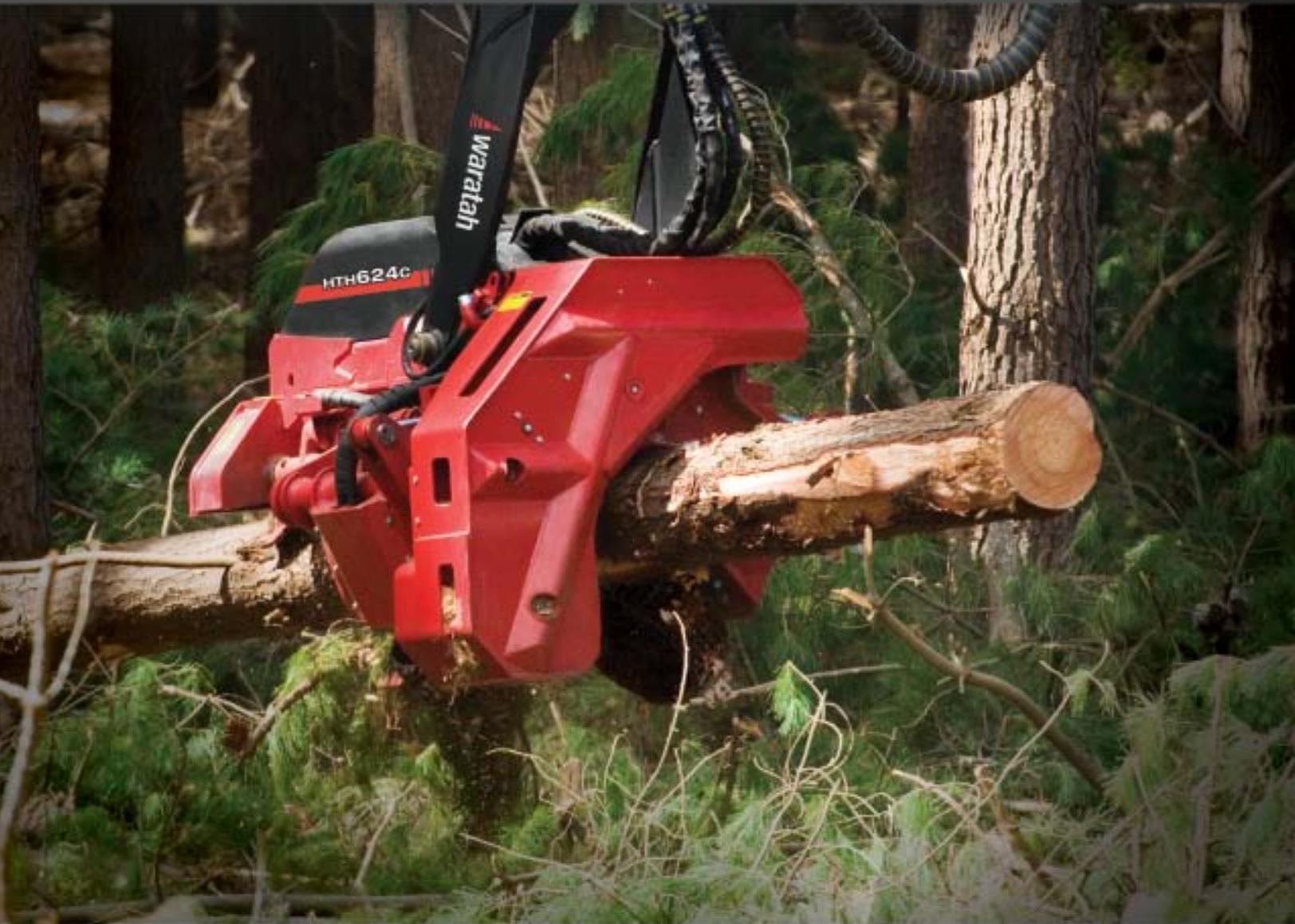
Proven in medium to large wood harvesting and processing, Waratah's big-timber-tackling HTH624C can easily handle species such as radiata pine, poplar, and aspen — up to 81 centimeters (32 inches) in diameter. With its rugged frame, large synchronized feed rollers, incredible drive power, and precision delimiting quality, it's a highly productive processor — whether you're working at a landing or felling and processing at the stump.
