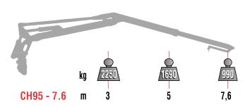
Actual lifting capacity depends on which link, rotator and harvester head is used.
