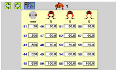
There are adjustment settings on the **Feeding Screen** for Feed Arms and Upper- and Lower-Delimb Knives, based on percentage available, so your operators do not need to be trained on the inner workings of this head to adjust its operation.
